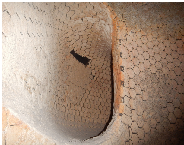
Figure 1. Failed refractory lining.
