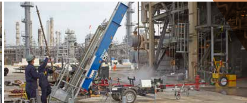
"The key is a basket at the end of the telescoping boom, able to lift 550 pounds of scaffolding up to 78 feet." ^
